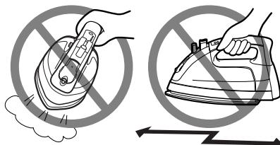
These actions can cause hot water to leak from the water inlet/outlet spout, resulting in possible burns.
